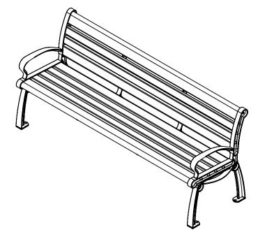
Tear drop board  $3.75" \times 1.34" 2.88"$  of flat surface on board Bull nosed board  $3.75" \times 1.34" 3.00"$  of flat surface on board Square board  $2.36" \times 1.34"$
