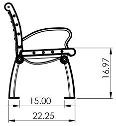
CONSTRUCTION MATERIALS: Recycled Plastic Cast Aluminum **HARDWARE:** Stainless Steel
